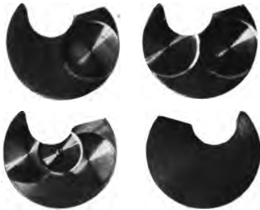
Fig. 9.—Showing Recessing and Facing of Top Plates.
