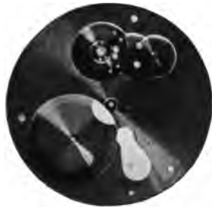
Fig 6.—Sixteen size Pillar Plate, showing six recesses made by Automatic Machine.
